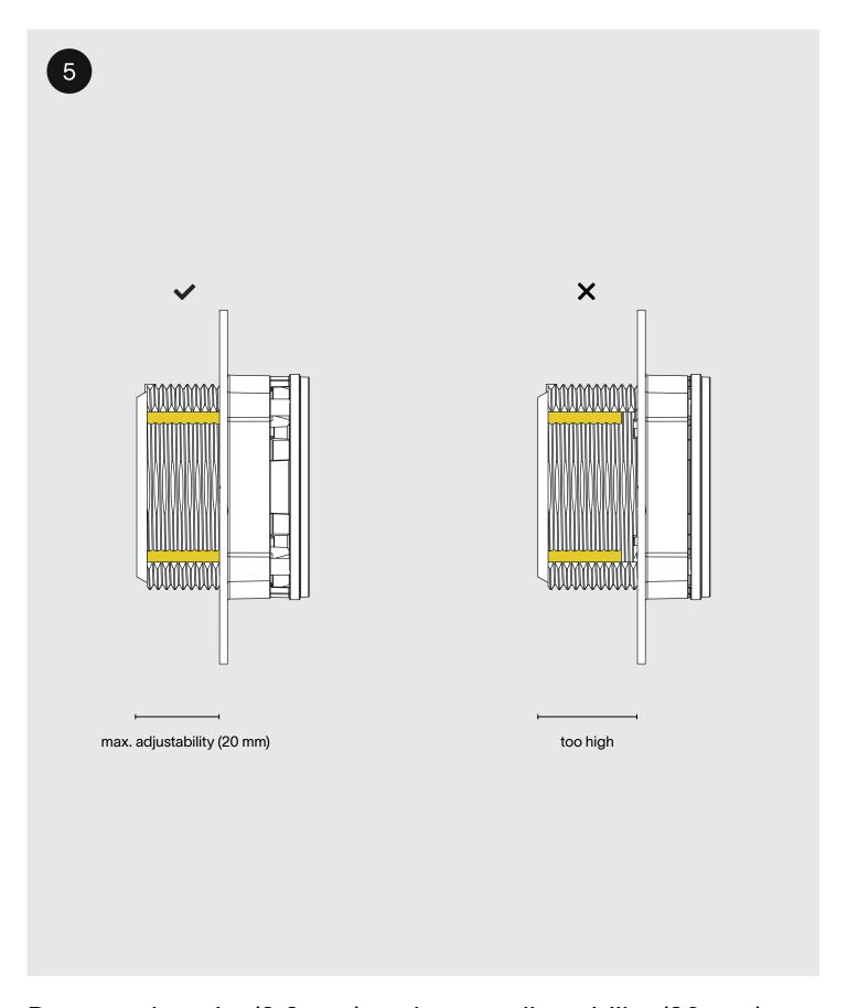
Respect the min. (3.6 mm) and max. adjustability (20 mm) when adjusting the height.
