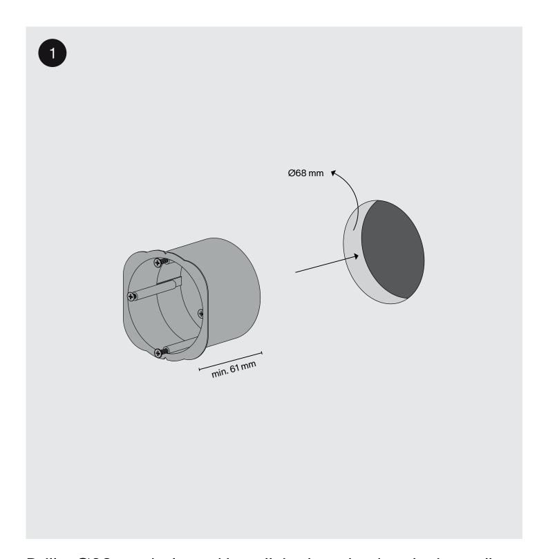
Drill a Ø68 mm hole and install the junction box in the wall.
