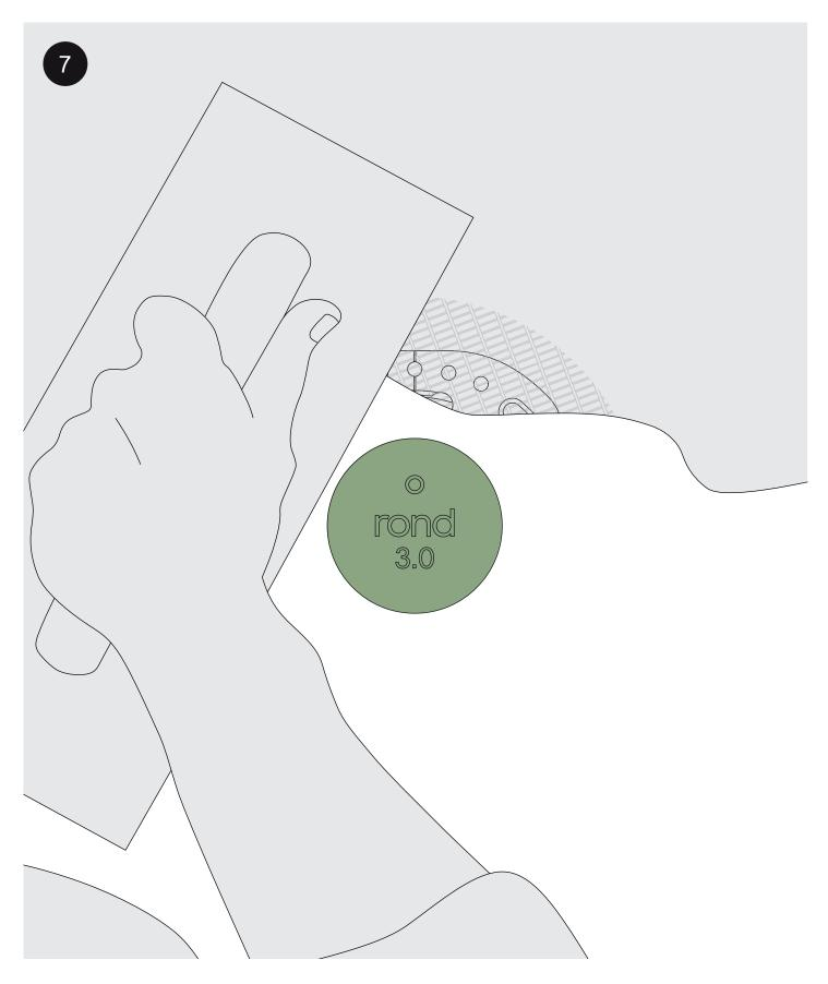
Excercise caution while plastering, do not damage the ring. Keep the plaster lid inside the mud ring while plastering.
