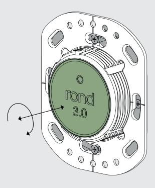
Remove the plaster lid and adjust the height of the ring to the desired plaster thickness by twisting the middle part.
