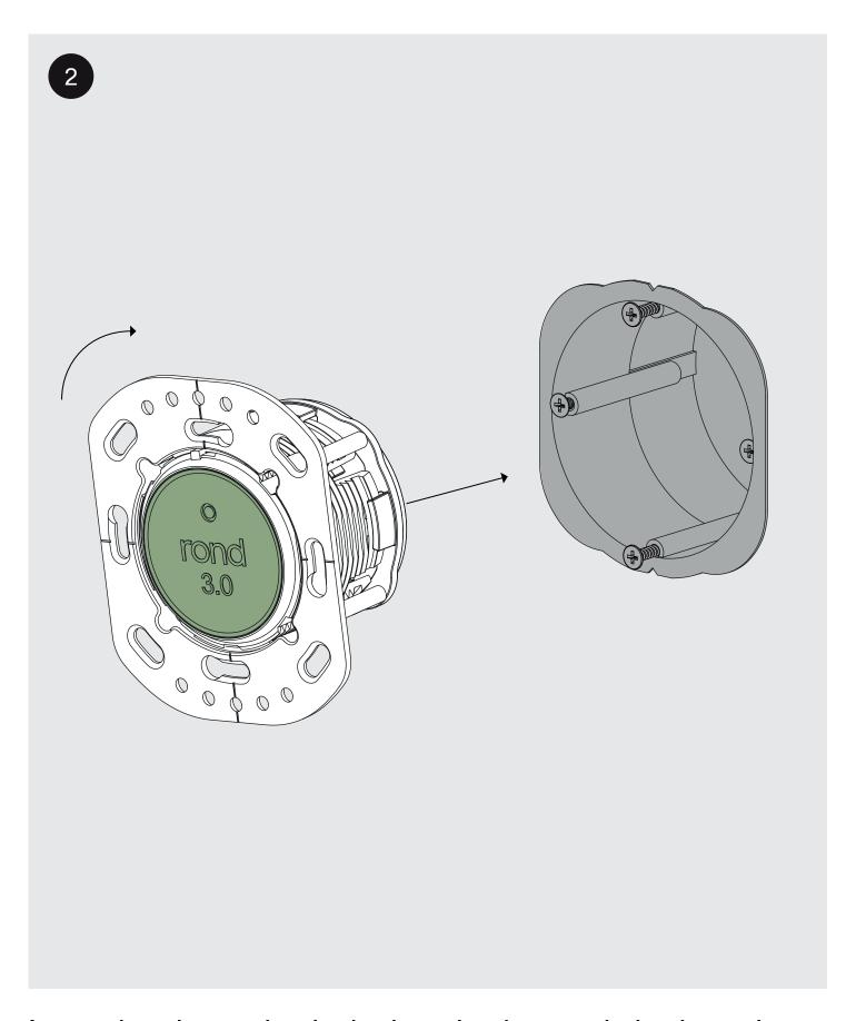
Insert the plaster ring in the junction box and give it a twist.
