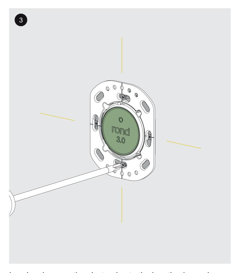
Level and secure the plaster ring to the junction box using the appropriate screws.
