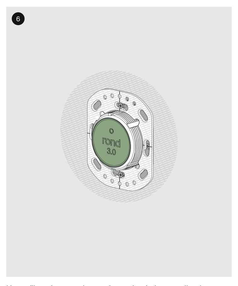
Use a fiberglass mesh tape for optimal plaster adhesion.
