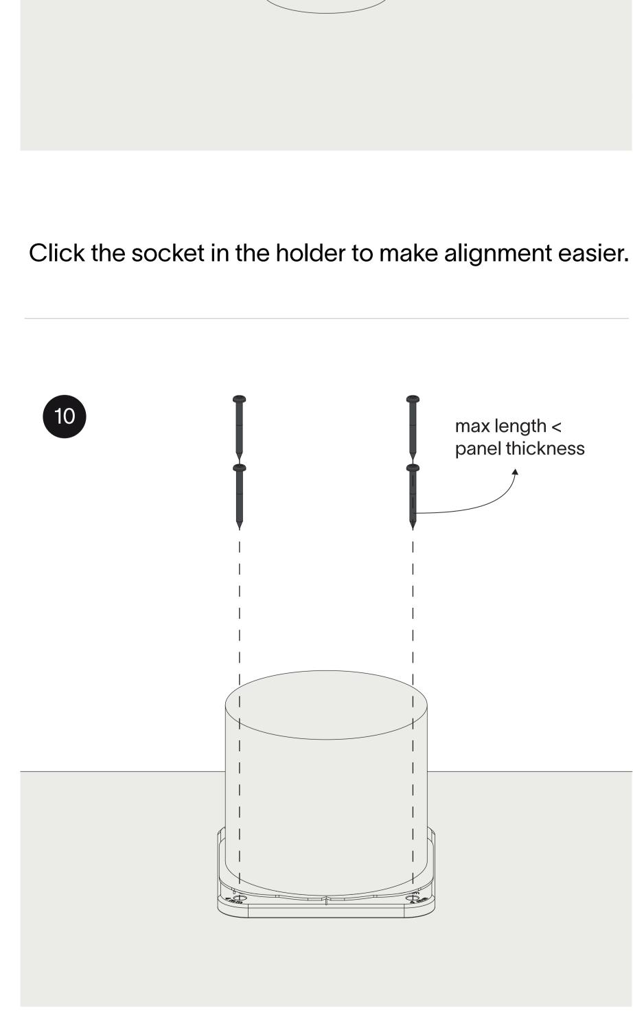
Fasten the backfit holder with junction box securely at
